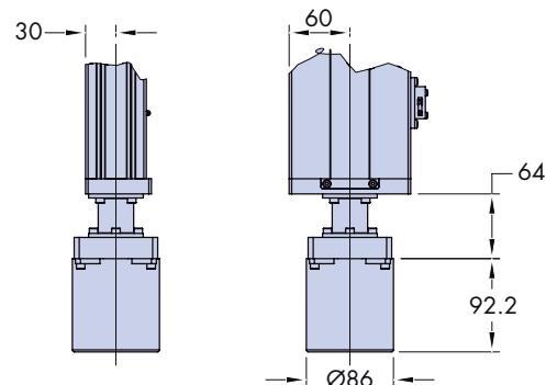
The fitted motor is a cost effective option, capable of high speeds and thrusts. Hepco can supply AC motors, stepper and servo systems including optional holding brakes, encoders for positioning and inverter drives for power and control.
