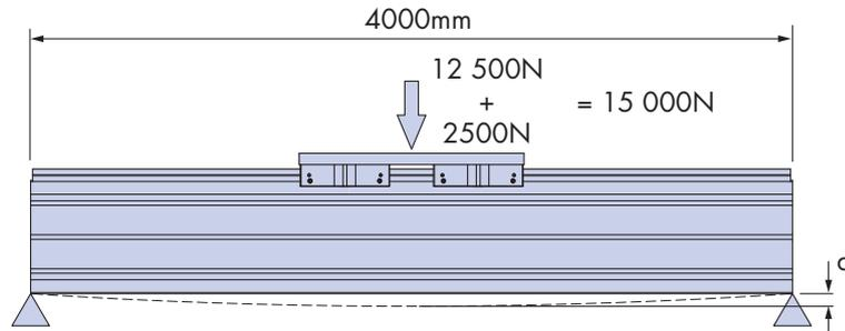
$$d = \frac{W \times L^3}{48 \times E \times I} \quad \text{equation 1}$$
