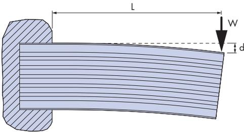
$$d = \frac{W \times L^3}{3 \times E \times I} \quad \text{equation 3}$$
