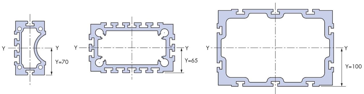
The beam deflection is accurately modelled by simple beam bending equations. The most common application is for a HDS2 construction beam supported at two points separated by a distance  $L$  (mm), subjected to a load acting at the midpoint of the span. The deflection  $d$  (mm) due to the applied load  $W$  (N) is measured adjacent to the point of loading. This is the worst case.
