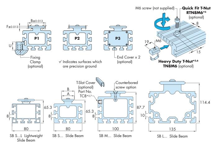
The counterbored Slide option is necessary if Slide Beams are to be used in conjunction with Belt Driven Carriages. This is to provide an uninterrupted path for the belt. Please see the GV3 Technical Guide 4.
