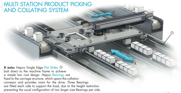
**Y axis:** Guidance for the product picking device is provided by Hepco Double Edge Spacer Slide with Fitted Rack ② to enable drive via a Hepco Pinion. The Slide runs in a "railway" of Controlled Height Twin Type Bearings 🕹 ③, which ensure alignment and compliance as the Slide engages. All Eccentric type Bearings are used except the two outermost on one side, which are the Concentric type in order to provide a datum for the system.
