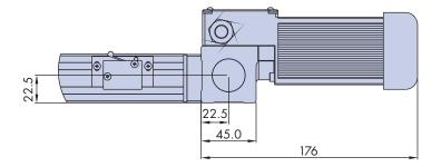
PDU2 AC geared motor shown mounted in position 5.
