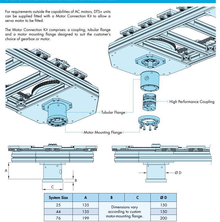
The dimensions of the custom motor-mounting flange will vary depending on the specification of motor that is selected. Dimensions are given in the table, above, to illustrate the size and layout of the Motor Connection Kit assembly. The table below details the coupling information for each system size, including the available bore diameters for the customer motor.
