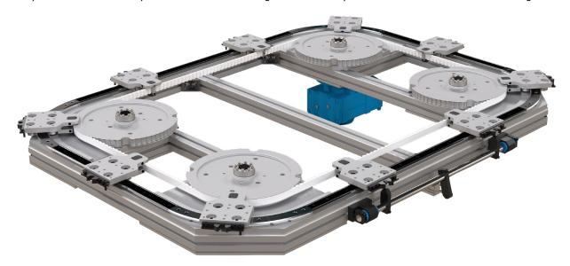
The DTS+ system incorporates key features of Hepco's PRT track system and original DTS, combining them with a high load capacity connection between carriages and the drive belt. The carriages will not disengage from the belt, allowing transmission of higher forces compared to the original DTS system.
