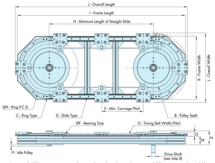
A system with 180° ring segments in an oval circuit is shown above. Rectangular systems with 90° segments are also available.
